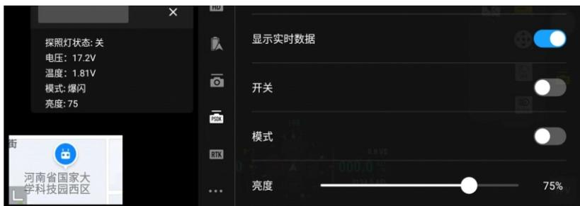
打开Payload设置，也可通过此菜单对探照灯进行操作（点击遥控器右上角菜单图标
